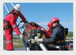
Bridge rope with a magnetic flux leakage testing instrument with roller system
